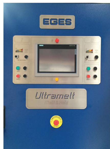
PLC & Converter Remote Control Cabinet
