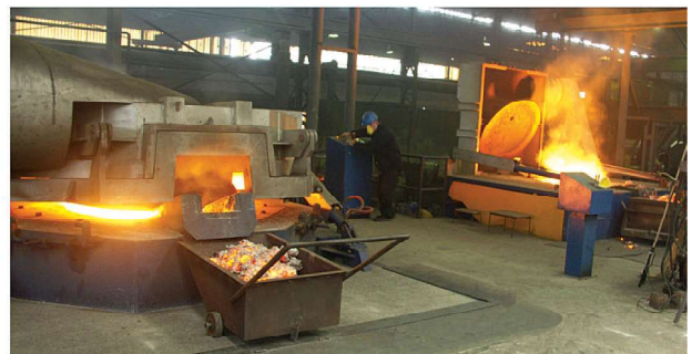
5 MW Melt&Hold 8ton+14ton Furnace System
