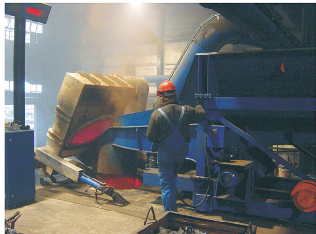
Charging By Vibrator Charger
