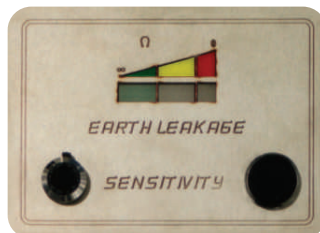
Earth Leakage Indicator
